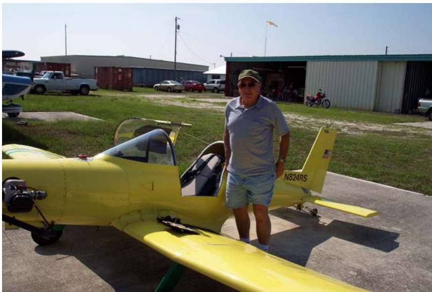
This is a Hummel Bird with half a VW engine. Hungry pilot flew up from Ft. Lauderdale area.
