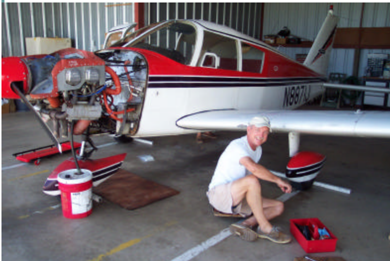
At Left -- Mike Ketchpaw is about to take off a main wheel as part of the Annual Inspeiton of the Flying Club's Cherokee.
